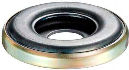
Worn spring strut support bearings should always be replaced by axle (i.e. on both sides of an axle at the same time). This prevents premature wear and reductions in safety and comfort. Well-known parts manufacturers are constantly analysing the causes of spring strut support bearing failure, using their findings to adapt the parts to meet the specific requirements of the prevailing application.
