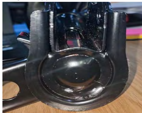
image 2: Appearance of the weld bead
